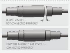
**IMPORTANT:** the 4 contacts connector should be connected properly so that the white o-ring is not visible and a clicking sound is heard.
