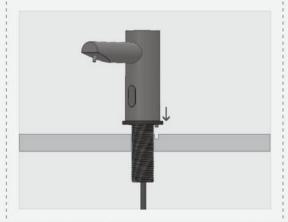
Under the deck, secure the gasket, disk and nut over the soap dispenser body nipple.
