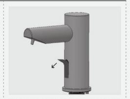
Connect the soap dispenser pump connector to its matching connector on the electronic unit. Please note that since the connector is waterproof, some pressure must be applied for a perfect seal.
